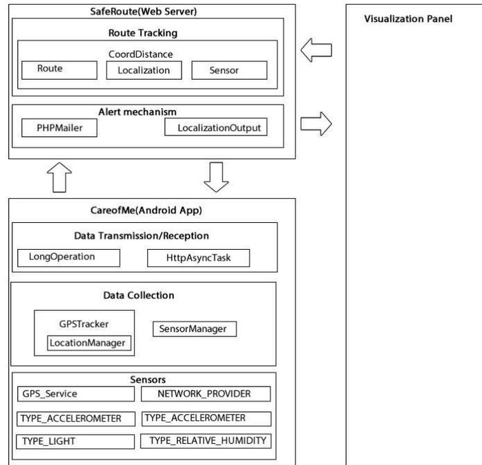
Fig. 2. SafeRoute system architecture.
