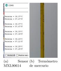
${\bf Fig.\,12.}\ {\bf Comparación\ del\ sensor\ MLX90614\ con\ un\ term\'ometro\ de\ mercurio.}$
