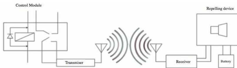
Fig. 6. Wireless remote control of a repelling device.
