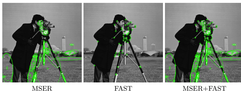
Fig. 2. Example showing the combination of two feature detectors (MSER and FAST) using the “cameraman” image.
