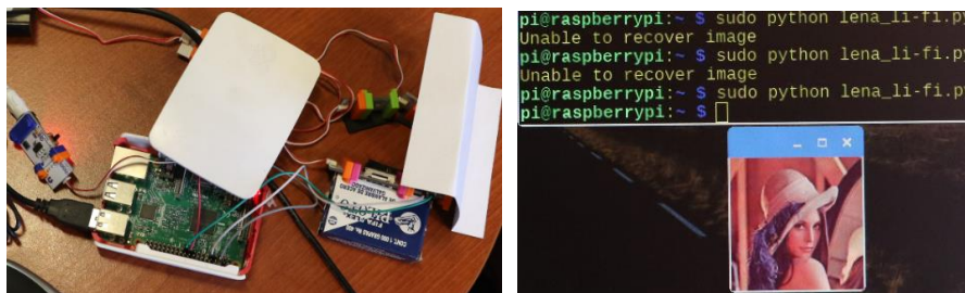
Fig. 13. Recovered picture via VLC after some adjustments.
