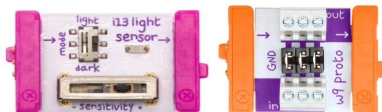
Fig. 6. Receiver components: Light sensor and proto bits.
