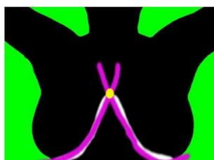
Fig. 8. Thinned line in white, curve fitting in purple and intersection point in yellow.
