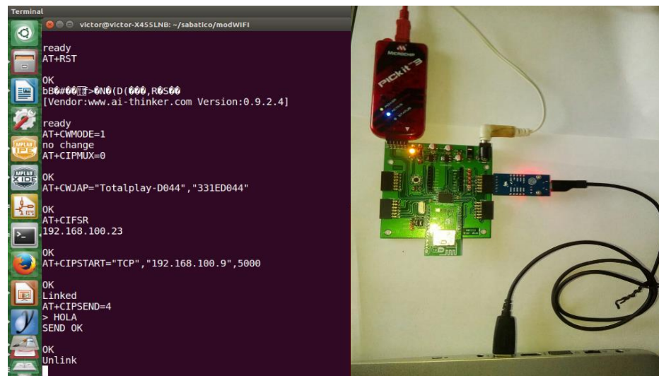
Fig. 5. Sensor node in operation with ESP8266EX.
