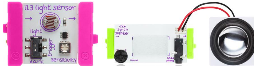
Fig. 5. Receiver components: Light sensor and speaker.
