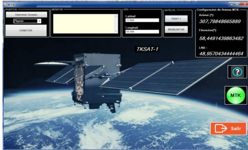
Fig. 8. Software user interface, application to calculate parameters of azimuth, elevation and polarization of LNB.
