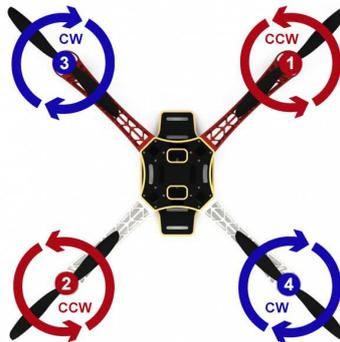
Fig. 1. Quad-rotor in X configuration.
