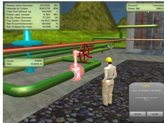
Fig. 6. Display System. Visor3D is responsible of rendering the virtual environment of the power plant
