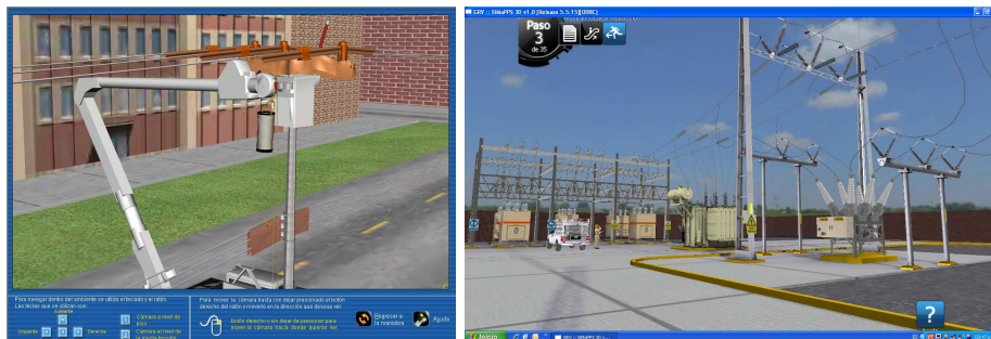
Fig. 5. Learning modes samples: medium tension live line maintenance (left) and substations primary equipment testing (right)
