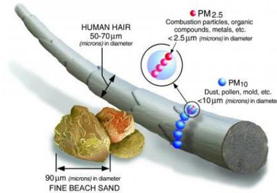
**Fig. 1.** Size of the PM<sub>10</sub> particle
