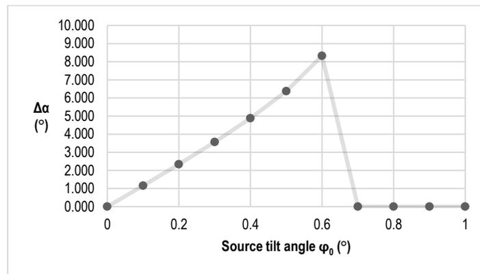
**Fig. 4.** The graph shows a lineal growth of the asymmetry in the output cone in the range between  $\phi_0 = 0.1^\circ:0.6^\circ$ , out of this range it is not possible determine te output angle in one of the marginal prisms, because for this cases the total internal reflection is presented.
