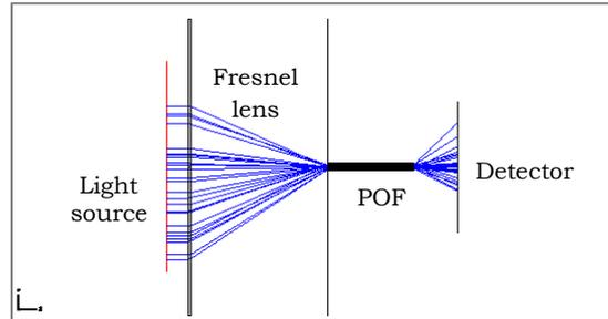
**Fig. 2.** Optical system design in Zemax OpticStudio®: the Fresnel lens has an output semi-angle of  $40.87^\circ$ , the POF has an acceptance semi-angle of  $27.23^\circ$ .
