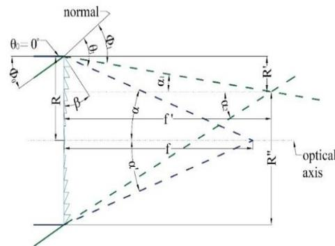
**Fig. 1.** Imaging Fresnel lens with grooves facing inward and source rays arriving parallel to optical axis,  $\theta_0$ , and other arriving with an angle  $\phi_0$ . The marginal rays for the 2 inputs generate 2 different output cones delimited by the marginal rays in each case.
