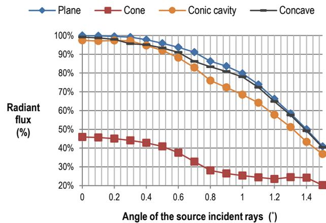
**Fig. 5.** Plane and concave FOP faces have better performance. The plane, concave and conic cavity fiber lenses show similar performance and have, in the theoretical critical tilt of the Fresnel lens ( $0.7^\circ$ ), efficiency around 80-90%.
