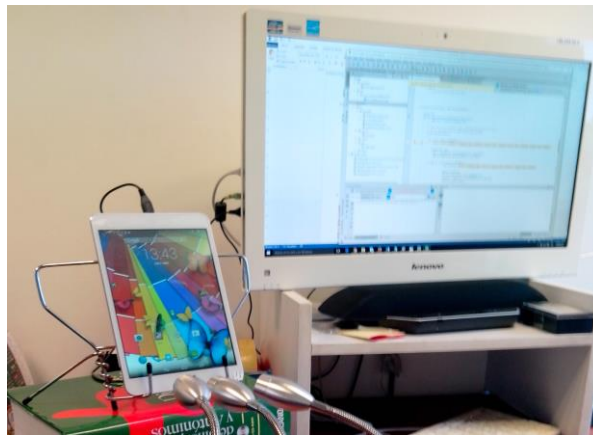
Fig. 9. GeoLiFi Kit Android Tablet 4.4.2 and three Li-Fi lamps.
