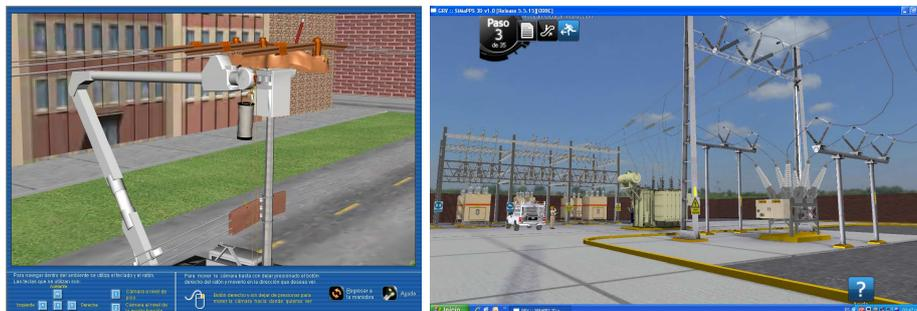
**Fig. 5.** Learning modes samples: medium tension live line maintenance (left) and substations primary equipment testing (right)
